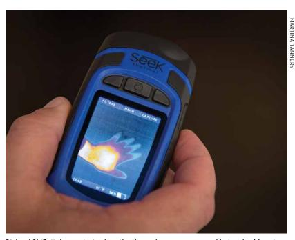
Richard Shiflett demonstrates how the thermal camera can reveal hot and cold spots created by something as simple as a quick handprint.
