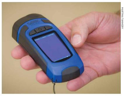
Tools like a thermal camera make a property manager's job easier. This one enabled members of Whitehall's team to find a water leak behind sprayed insulation in an attic.
